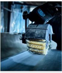
**TYROLIT Power** revolutionised the finishing of hard surfaces. Sanding strips consisting of layers made from cactus hair and diamond provide extreme hardness, save time and significantly reduce vibrations for the user.
